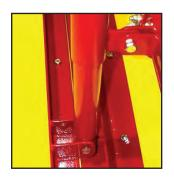
**STEP 2:** Attach the raise/lower JACK to the tabs at the front of the compactor (3/8" x 2-3/4" hex bolt and locknut), and on the cross piece of the drawbar (3/8" x 1-1/4" hex bolt and locknut).
