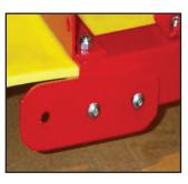
STEP 3: Attach the two steel skid plates to the rear corners of the compactor bed with two 5/16" x 3/4" button head socket screws on each. NOTE: that the plates can be rotated
