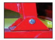
**STEP 1:** Attach the drawbar to the compactor using 3/8" x 2-3/4" hex bolts and locknuts.
