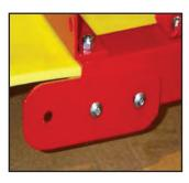
STEP 3: Attach the two steel skid plates to the rear corners of the compactor bed with two 5/16" x 3/4" button head socket screws on each. NOTE: that the plates can be rotated
