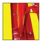
**STEP 2:** Attach the raise/lower JACK to the tabs at the front of the compactor (3/8" x 3-1/4" hex bolt and locknut), and on the cross piece of the drawbar (3/8" x 1-1/4" hex bolt and locknut).
