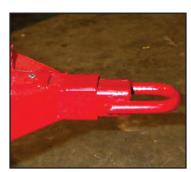
STEP 4: Insert the hitch in the drawbar and fix with an 8 penny nail. Bend the nail over on the underside of the drawbar to prevent any injury when handling. See the operation section of this manual for more information on shear pins.
