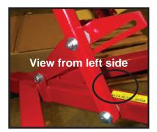
STEP 2. Bolt the Lever Arm to the square tube behind the hitch point  $(3/8" \times 3-1/2")$  hex bolt for one lift lever, 4-1/2" hex bolt for double lift levers on the six foot model – we supply both bolts, you will select only one. Bolt the slotted hook plate to the upright tab on the front point of the drawbar  $(5/16" \times 1")$ . Note: If you are installing double lift levers, one will
