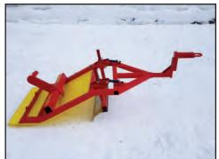
**loop hitch** to the hitch extension. Note that you can place the hitch with the channel pointing up or down, depending on the desired height needed to mate with your tow vehicle. The carriage bolts go in from the rear of the plate with the square slot.
