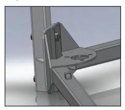
Remove your old hitch from the front of the G2. Assemble the main "L" shaped part of the Gooseneck Hitch, channel backing plate, (2) 1/2" x 3-3/4" hex bolts and (2) 1/2" lock nuts as shown in the picture, and tighten securely.
