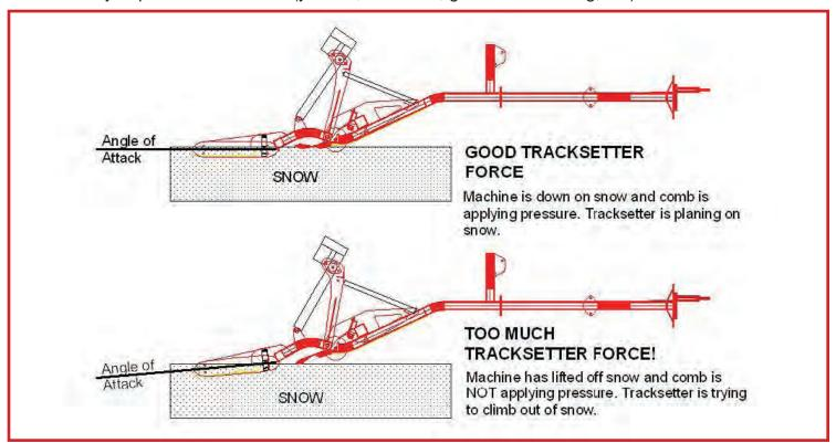
Lesson: Make sure that your G2 comb is always FULLY FLEXED, and the Tracksetter is not forcing the comb up off of the snow!
