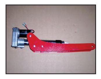
Assemble the three main components as shown in the pictures, using the  $\frac{1}{2}$ " x 6" Hex Bolt, bronze bushings and the locknut. The lock nut need only be tightened to the point that it engages the nylon lock-
