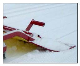
damage the machine, but may jiggle your tracks. It is not recommended that you hit objects closer than 6" in from the end of the flaps – you could bend the flap arm. If this does happen, you can straighten the arm and reattach. Don't forget that you can run the side flaps with one up and one down – sometimes a solution when you are trying to renovate close to a set track and not disturb it.
