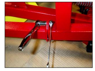
bolt provided in the actuator clevis. Swing the actuator up into place on the "rollbar" portion of the rear frame, placing the trunnions (short round pegs) on each side of the actuator cylinder into the 1/2" flange bearings (included with actuator) and attach using fasteners provided. NOTE – you may find it helpful to place block under the toothbar
