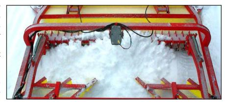
the blades and the teeth. A little bit of snow may pass over the teeth, but you should not allow the snow to accumulate to the point that it starts to pass over the compactor bed or outward around the sides of the toothbar. The blades also help fill depressions and aid in leveling.
