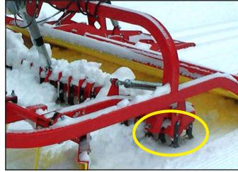
when the job is tough, it is usually more efficient to make multiple light passes than one single slow heavy pass. Also remember that it is neither necessary nor desirable to always renovate as deeply as possible. Often, the best product results from just barely scratching the trail surface.
