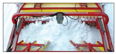
the blades and the teeth. A little bit of snow may pass over the teeth, but you should not allow the snow to accumulate to the point that it starts to pass over the compactor bed or outward around the sides of the toothbar. The blades also help fill depressions and aid in leveling.
