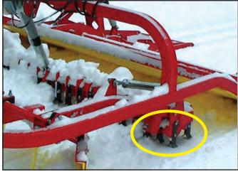
when the job is tough, it is usually more efficient to make multiple light passes than one single slow heavy pass. Also remember that it is neither necessary nor desirable to always renovate as deeply as possible. Often, the best product results from just barely scratching the trail surface.
