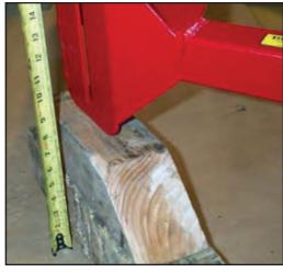
to get it at the right height to line up the holes in the flange bearings. AGAIN – watch those sharp teeth! Block up the front of the frame under the hitch plate to a height of about 7 1/2". Check to see that the frame is close to level, and if not, adjust the blocking. Just get it within 1/2"...
