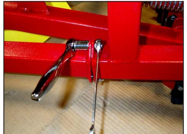
bolt provided in the actuator clevis. Swing the actuator up into place on the “rollbar” portion of the rear frame, placing the trunnions (short round pegs) on each side of the actuator cylinder into the 1/2” flange bearings (included with actuator) and attach using fasteners provided. NOTE – you may find it helpful to place
