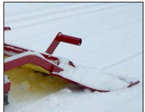
damage the machine, but may jiggle your tracks. It is not recommended that you hit objects closer than 6" in from the end of the flaps – you could bend the flap arm. If this does happen, you can straighten the arm and reattach. Don't forget that you can run the side flaps with one up and one down – sometimes a solution when you are trying to renovate close to a set track and not disturb it.
