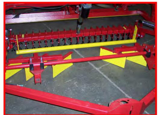
removing more air. This enhances surface compaction and side to side levelling. Lastly, consistent depth of cut creates greater efficiency by reducing drag on your tow vehicle.
