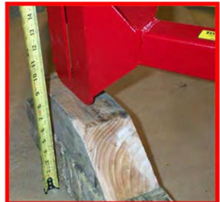
Block up the front of the frame under the hitch plate to a height of about 7 1/2". Check to see that the frame is close to level, and if not, adjust the blocking. Just get it within 1/2"...
