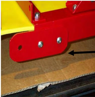
STEP 3. Attach the two steel **skid plates** to the rear corners of the compactor bed with two 5/16 x 3/4" button head socket screws on each. **NOTE:** that the plates can be rotated in four positions after they have worn down due to dragging the machine on dirt or pavement. Make sure to call us and order replacement skid plates before you wear into the bolt holes.
