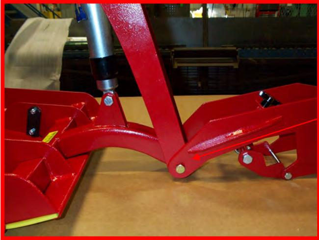
1/2x6 bolt, with lock nut through three assemblies. DO NOT OVERTIGHTEN! Just engage lock nut threads securely.
