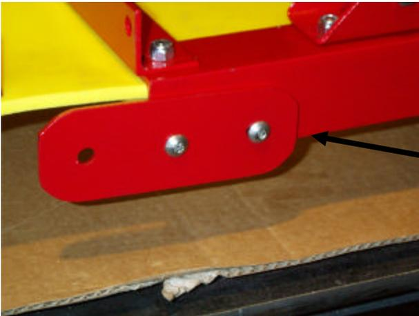
STEP 3. Attach the two steel **skid plates** to the rear corners of the compactor bed with two 5/16 x 3/4" button head socket screws on each. Note that the plates can be rotated in four positions after they have worn down due to dragging the machine on dirt or pavement. Make sure to call us and order replacement skid plates before you wear into the bolt holes.
