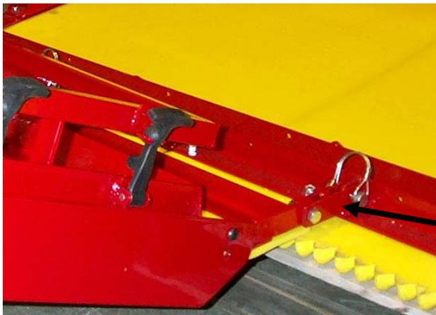
**STEP 3.** Bolt the **link arms** on the front tabs using 3/8 x 1-1/4 hex bolts and locknuts (do not tighten to the point that you deform the link). Attach the track setter to the rear edge of the compactor comb using the clip pins provided.
