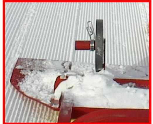
This is the recommended way to add weight to the G2. You may want to experiment with various amounts of weight and/or Tracksetter gas spring combinations (see the Tracksetter section) in different conditions on your terrain and with your snow machine. In theory, you get better compaction with more weight, but the trade off is the increased pulling power needed to get up hills.
