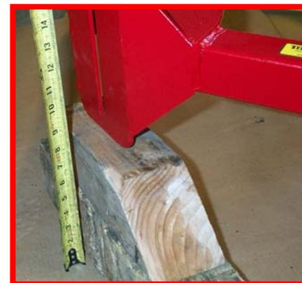
Block up the front of the frame under the hitch plate to a height of about 7 1/2". Check to see that the frame is close to level, and if not, adjust the blocking. Just get it within 1/2"...
