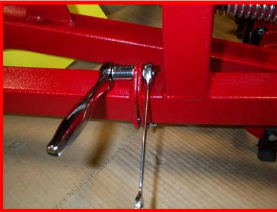
Move the rear frame member (with yellow plastic bed and attached comb) into place behind the front frame member. Using the bolts already in place, join the two frame members together and tighten the bolts and nuts with 9/16" wrenches.
