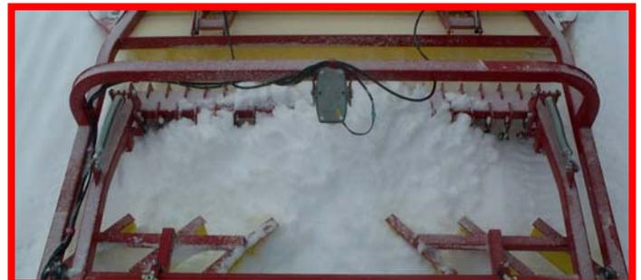
snow to accumulate to the point that it starts to pass over the compactor bed or outward around the sides of the toothbar. The blades also help fill depressions and aid in leveling.
